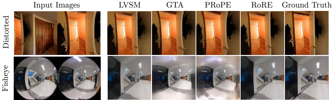
Figure 3: Qualitative results on distorted and fisheye inputs. RoRE preserves scene structure under both barrel-distorted perspective images (top) and native fisheye images (bottom), whereas competing methods produce severe artefacts or fail to reconstruct meaningful views.
